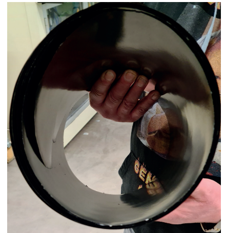
Fig. 1. By modifying the highly filled plastics, considerably thinner bipolar plate films can be produced than was previously the case © Eisenhuth
